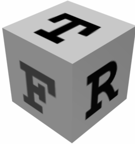
-Figure 5- Example of one base mesh that would require several texture meshes. The "T", "R", and "F" quads are each textured with a different bitmap, and the texture coordinates are not contiguous.
